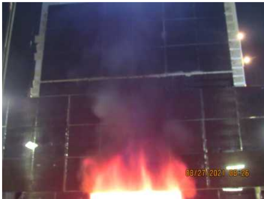
Photo No. 4 Flames Exiting Window
