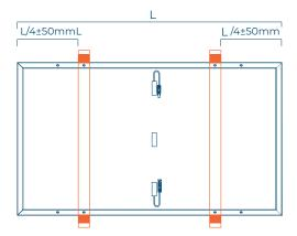
Front Static Load 5400 Pa, Rear Static Load 5400 Pa
