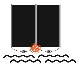
WARNING: Ensure cabling is adequately protected from direct sunlight, dirt, debris, moisture, and mechanical friction.
