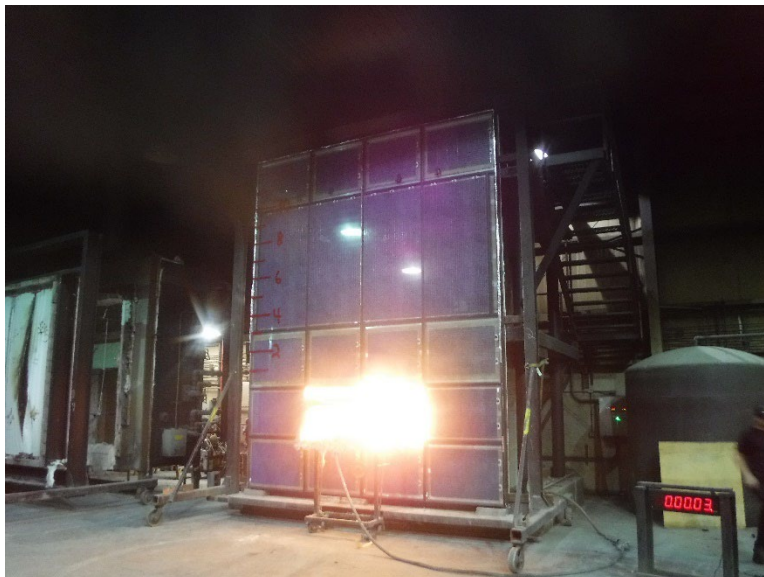
Photo No. 12 Ignition of Room Burner
