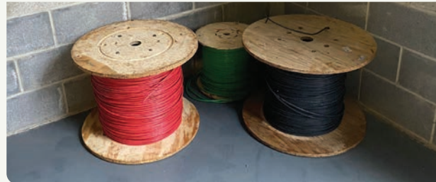
Wires - DC cable for panel connection.
