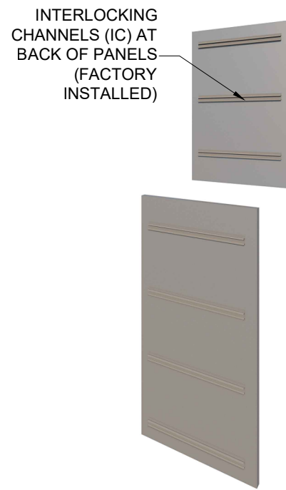
STEP 08 : INTERLOCKING CHANNEL (IC) TO BACK OF PANEL
