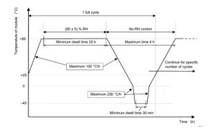
MQT 13 Damp Heat Test
