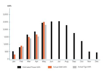
Since the total DC size of system is 36 kW, the specific production (Performance index) of this project is 513 kWh/kWp/Year (equal to 513 hours).
