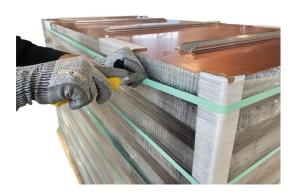
9. Using the protective corner cardboard pieces as support, cut the plastic film at the same height of 2 panels.
