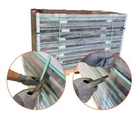
8 Cut only the first horizontal strap (4.). Make sure you do not cut or damage the honeycomb or glass facing.
