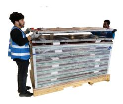
**WARNING:** The glass facing of the module can be damaged if it is not placed properly. Make sure that if the panel is facing down, there is not any screw or metallic piece that can damage the surface.
