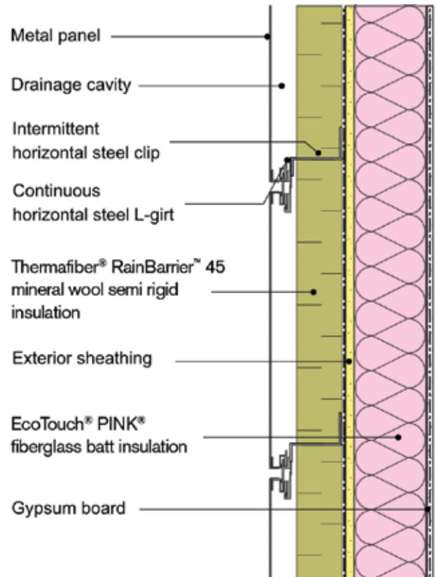
**Table 5.2: Thermal Transmittance Data for Detail 2**
