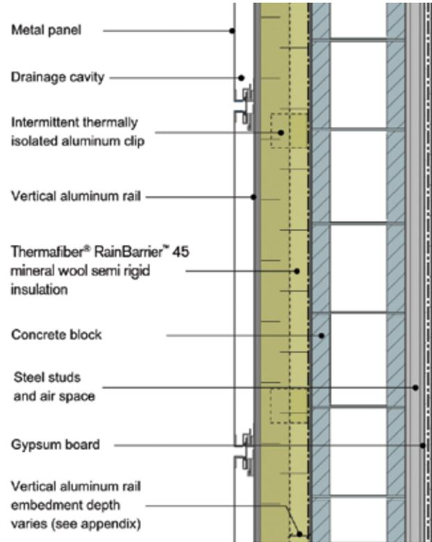
**Table 5.6: Thermal Transmittance Data for Detail 6**
