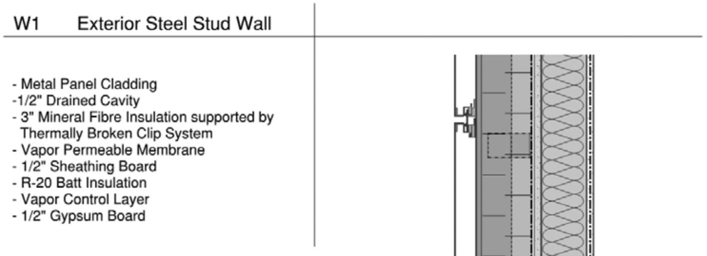
**Example Steel Stud Wall Assembly Drawing**
