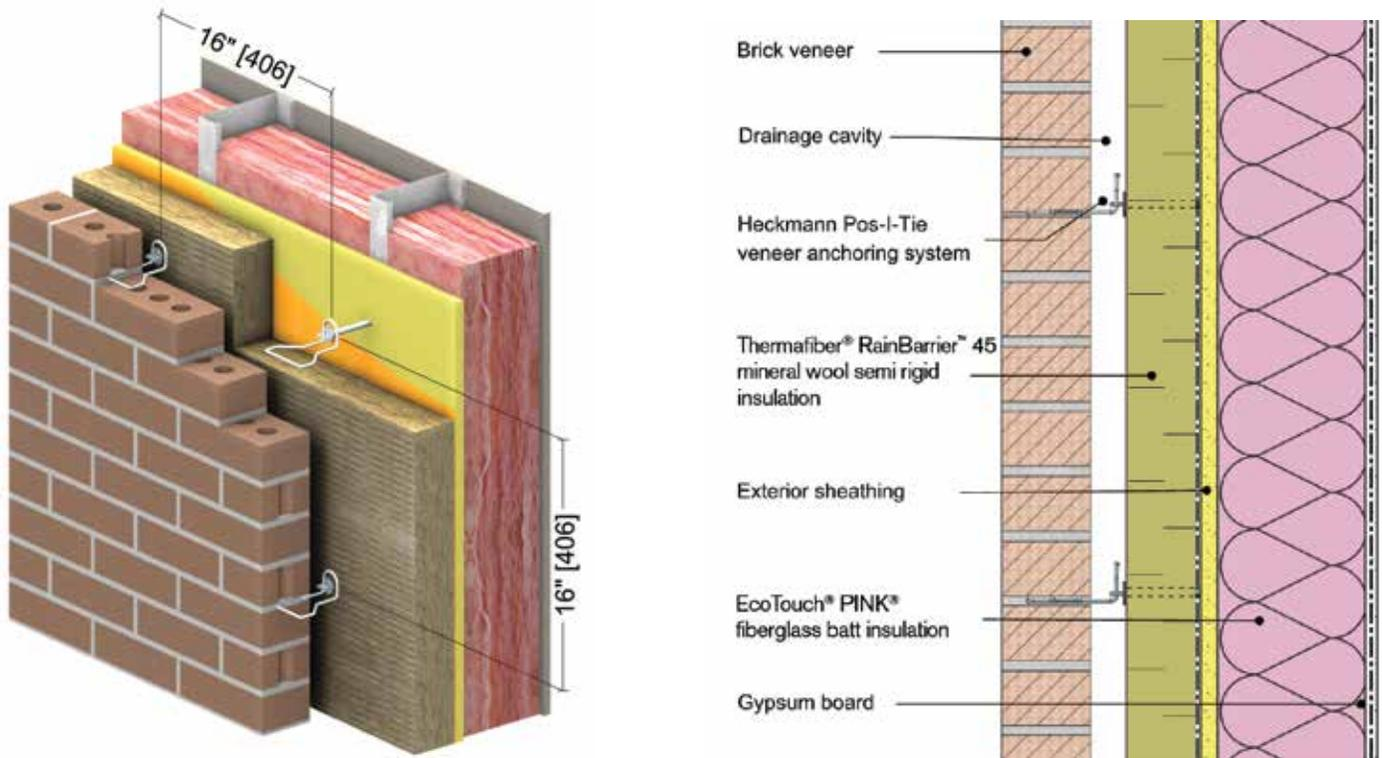
Table 5.4: Thermal Transmittance Data for Detail 4
