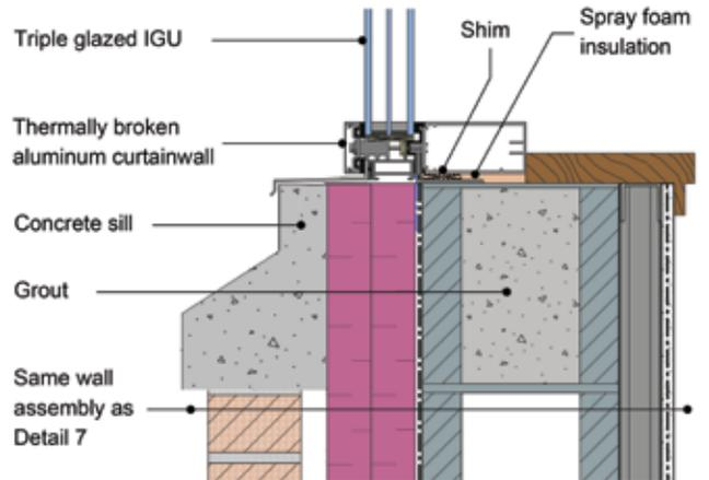
**Table 5.14: Thermal Transmittance Data for Detail 14**
