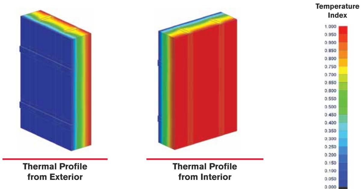
(3" Exterior Insulation and R-20 Batt Insulation scenario shown)
