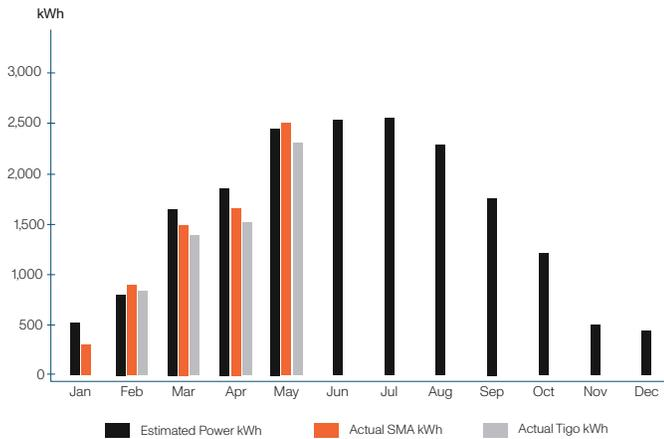
Since the total DC size of system is 36 kW, the specific production (Performance index) of this project is 513 kWh/kWp/Year (equal to 513 hours).
